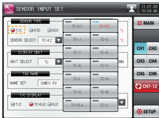
[Fig. 13-4] Screen for selecting the T/C sensor type
