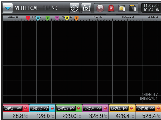
[Fig. 4-1] Screen when the graph is not saved (Black screen)
