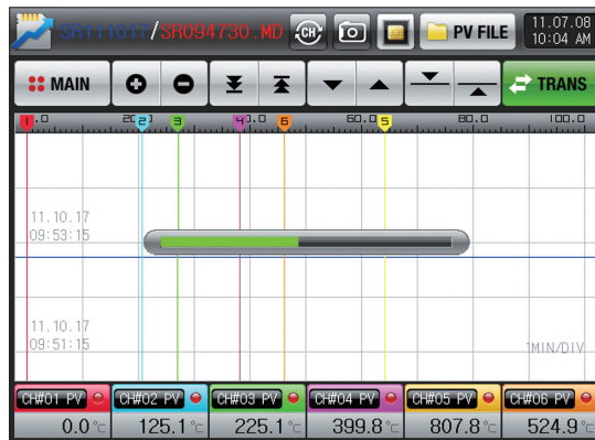
[Fig. 5-7] Screen for PV graph transmitting which is opened currently
