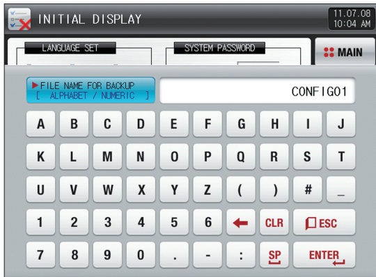
[Fig. 18-7] File name setting for transmission to SD cards
