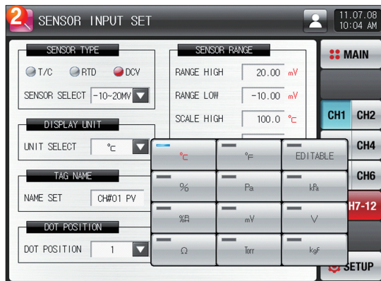
[Fig. 13-9] Screen for setting the DVC sensor display unit
