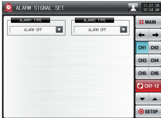
[Fig. 14-2] Alarm signal setting screen 2 #1
