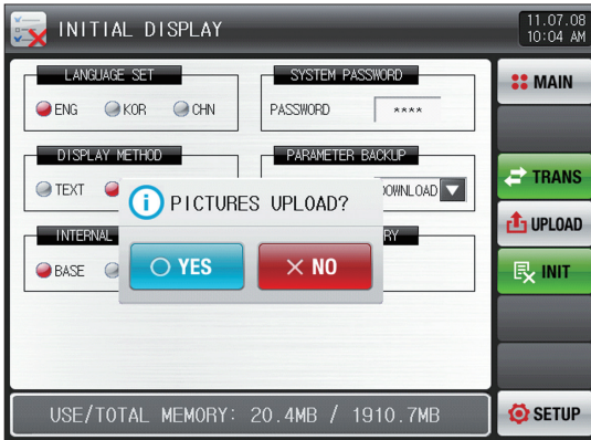
[Fig. 18-3] Upload the file saved in SD card into internal memory
