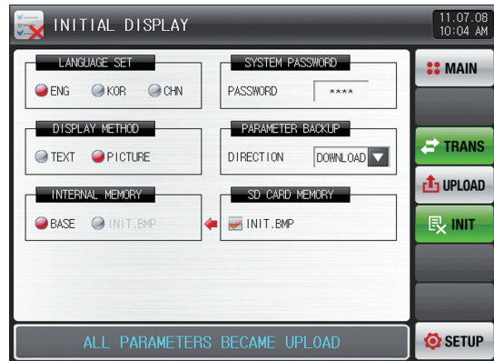
[Fig. 18-13] Screen after sending the saved parameter in the SD card to SDR
