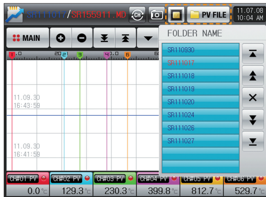
[Fig 5-2] Opening the PV file (Selection of the folder in internal memory)
