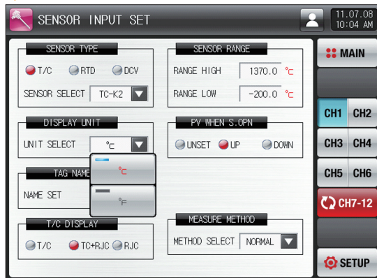
[Fig. 13-5] Screen for setting the T/C sensor display unit
