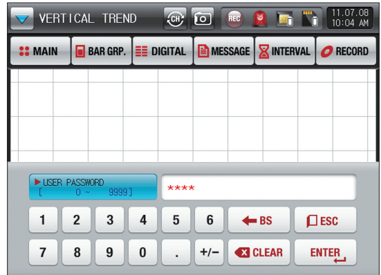
[Fig. 6-7] Screen for setting the main button restriction
