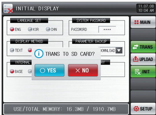
[Fig. 18-6] Parameters transmission setting from SDR to SD cards
