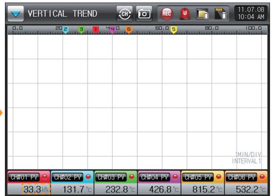
[Fig. 13-14] When the graph screen is kWh setting
