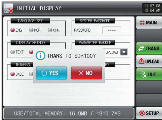
[Fig. 18-10] Screen setting for sending the parameter saved in the SD card to SDR
