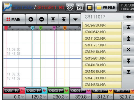
[Fig 5-3] Opening the PV file (Selection of the file in internal memory)
