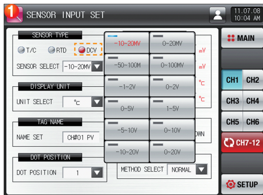
[Fig. 13-8] Screen for selecting the DVC sensor type
