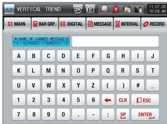
[Fig. 4-8] The screen selected with EDIT NEW MESSAGE in message input
