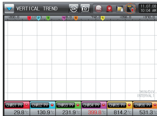
[Fig. 6-4] The screen not available for saving due to no space in memory on the card
