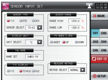
[Fig. 13-1] Sensor setting screen (T/C)
