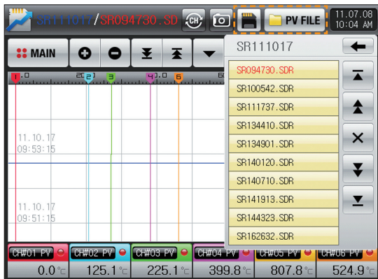
[Fig. 5-5] PV file open (Selection of the file stored in the SD)
