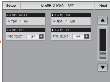
[Fig. 7-3] Alarm signal selection #1 in screen 2
