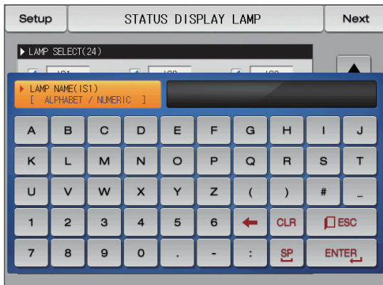
[Fig. 12-6] setting screen for lamp name
