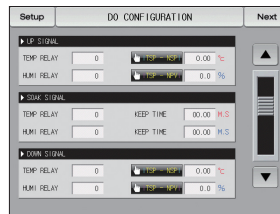
[Fig. 10-9] Sub output relay setting screen #2
