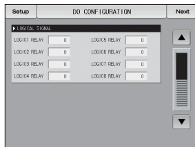
[Fig.10-7] Logical signal relay setting screen
